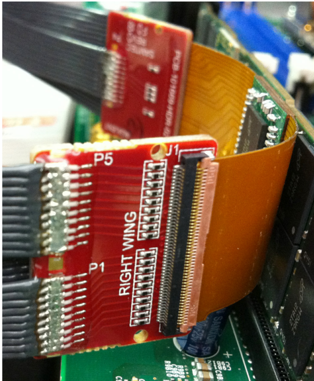
Figure 15a and 15b. W4633A x4/x8, 3-wing BGA interposer with two E5849A DDR4 ZIF probes attached. Note that the ZIF door closes on the bottom side of the wings. This is true for both the W4633A and W4631A DDR4 BGA interposers.
