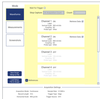
The setup window enables the selection of the Waveforms, Measurements, or Screenshots mode.
