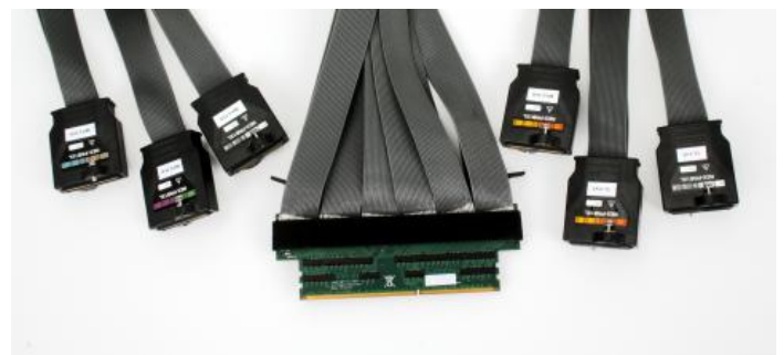
TLA Logic Analyzer and Probes for multichannel signal capture
