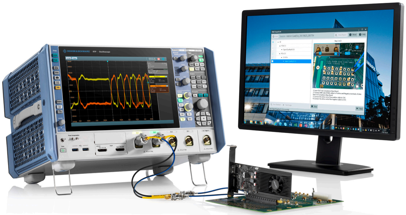
Automated PCI Express compliance test
