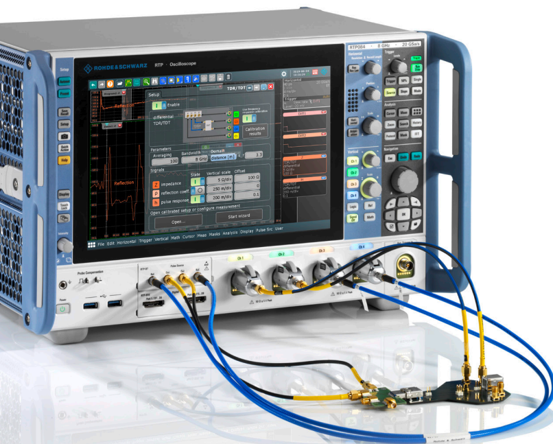
TDR/TDT wizard supports setup, calibration and analysis
