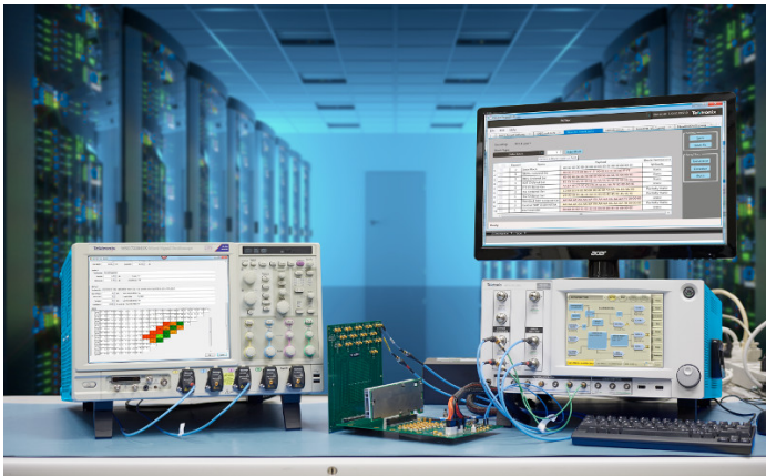
PCIe receiver test setup
