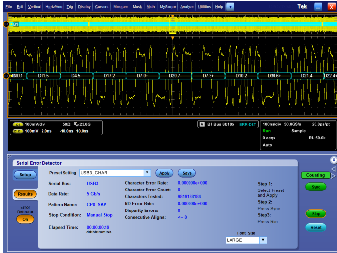
Testing CP0 compliance pattern with Tektronix Scope Error Detector
