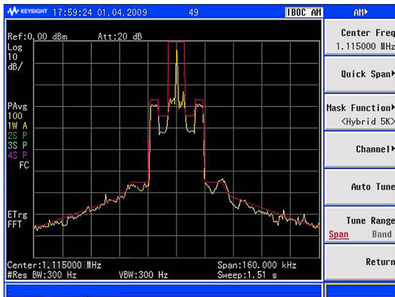
IBOC-AM measurement with N9340B IBC
