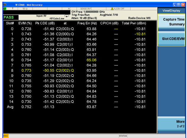
Figure 8. HSUPA capture time summary trace showing error metrics for 15 consecutive slots
