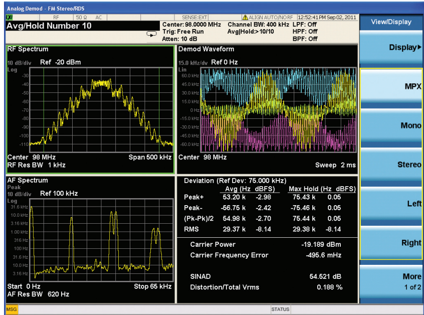
Figure 6. FM stereo MPX view/display with RF spectrum, AF spectrum, demod waveform and demodulation metrics results.
