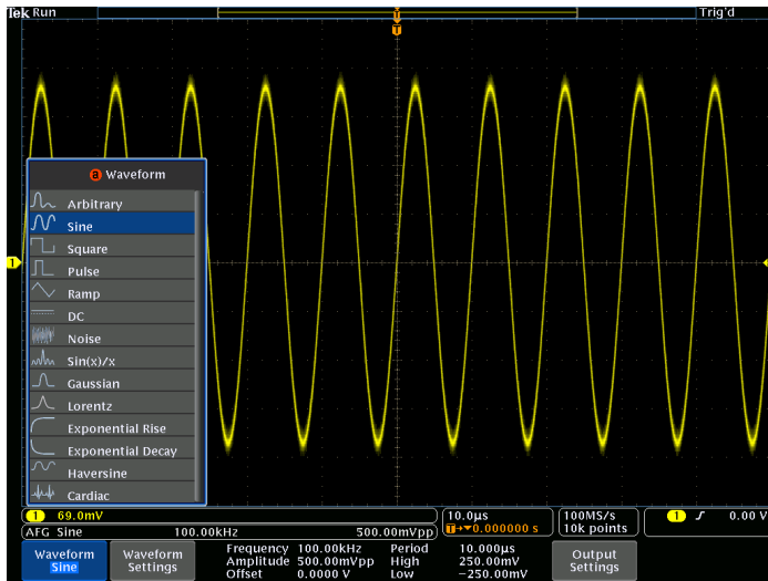
Waveform type selection in the integrated AFG.
