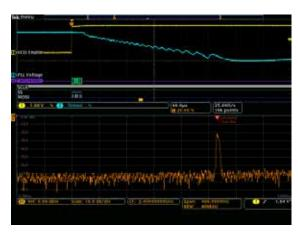
2. Spectrum Time is moved about 90  $\mu$ s to the right. At this point, the spectrum shows that the PLL is in the process of tuning to the correct frequency (2.400 GHz). It has made it down to 2.4924 GHz.
