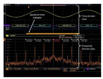
The upper half of the MDO4000C Series display shows the Time Domain view of the analog and digital channels, while the lower half shows the Frequency Domain view of the spectrum analyzer channel. The orange bar – Spectrum Time – shows the period of time used to calculate the RF spectrum.
