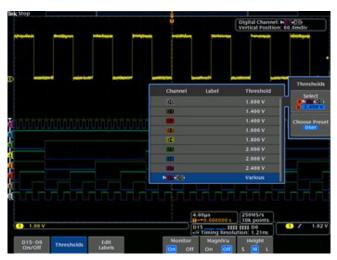
With color-coded digital waveform display, groups are created by simply placing digital channels together on the screen, allowing digital channels to be moved as a group.
