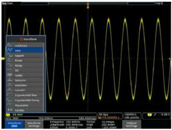
Waveform type selection in the integrated AFG.
