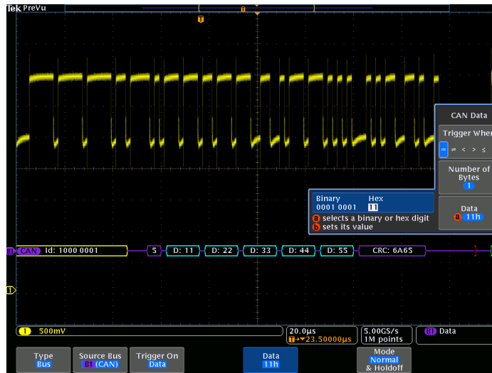
Triggering on a specific data value on the CAN bus.
