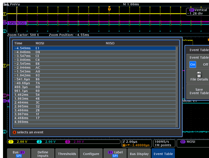
Event table for SPI bus with all captured packets time stamped and in a tabular view.
