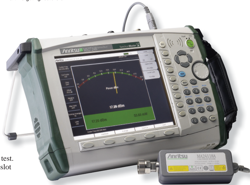
MA24118A with MS2724B Spectrum Master
