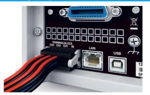
To facilitate typical calibration setups, the rear panel connector was designed with a WAGO cage clamp.
