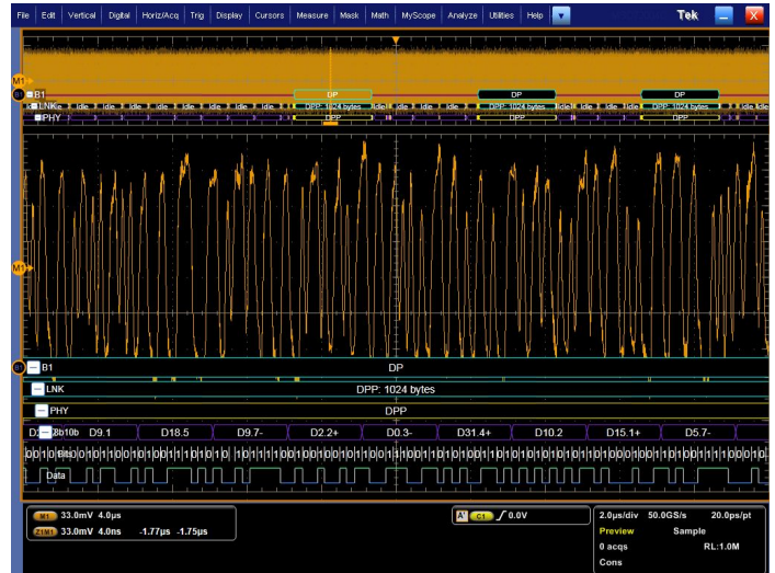
USB 3.0 bus display showing multiple layers simultaneously
