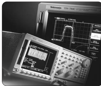
▶ The AWG520 can easily generate telecom signals which complement masks from a digital oscilloscope.
