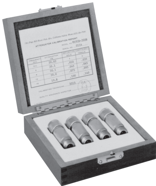
Figure 7. Coaxial fixed attenuator set
