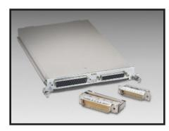
The Model 7701 plug-in module offers 32 channels of 2-pole or 16 channels of 4-pole multiplexer switching. Its 32 channels can be configured for common-side 4-wire ohms. They can also be configured as two independent banks of multiplexers. It is ideal for RTD or thermistor temperature applications.
