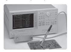
The 42941A impedance probe enables in-circuit impedance measurement of electronic circuits or components. Grounded devices can also be measured.
