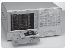
The 42942A terminal adapter converts the four-terminal-pair port configuration to an 7-mm port. This adapter permits the use of familiar 7-mm test fixtures.
